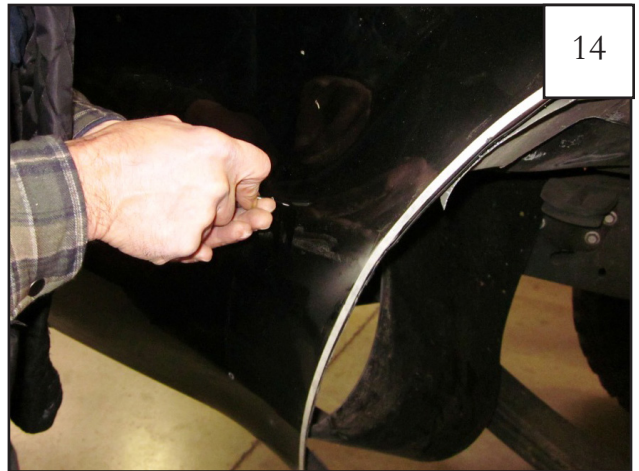
Remove flare. Using marks made with scratch awl as a guide, score the sheet metal with a center punch prior to drilling.
