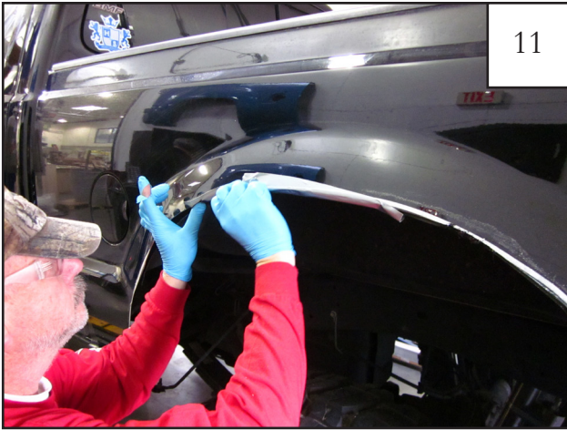
If needed, use tape to prevent caulk from dripping while drying.
