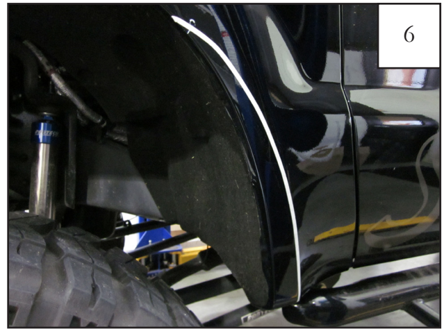
Using marks as a guide, use masking tape to create an arc from the lower mark to the upper mark. Inner edge of tape should be outside of marks made in previous step.
