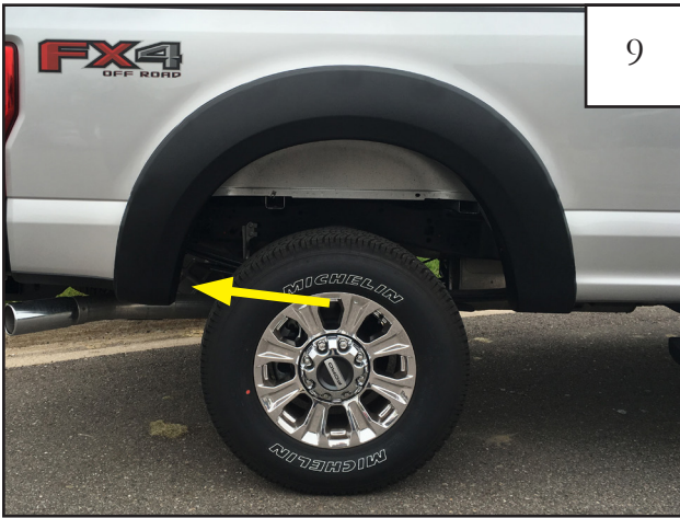
Install supplied push retainer (RV1-P0001) into flare and through factory hole at rear of wheel well.
