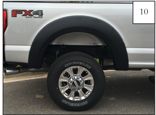
Completed rear flare installation.
