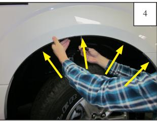
Using a 7mm socket wrench, reinstall the factory screws through the inner piece.
