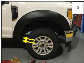
Still holding flare to fender, re-install remaining factory screws removed in Step 1 using 7mm socket and wrench. Tighten all screws.
