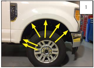
Remove six factory screws with a 7mm socket wrench. Save screws for reinstallation.
