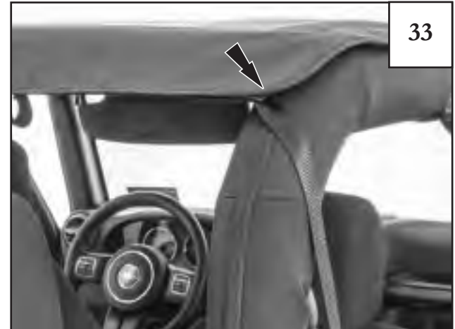
Locate the long strap at the rear corner of the main deck. Pull it straight and to the outside of the sport bar.
