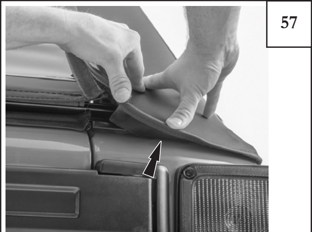
Clip in the last portion of window corner under the rear window retainers as shown.
