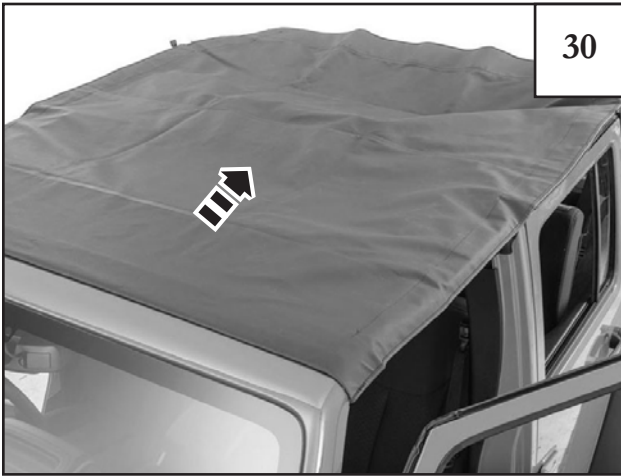
Un-Fold the soft top over the sport bar frame working toward the rear of vehicle.
