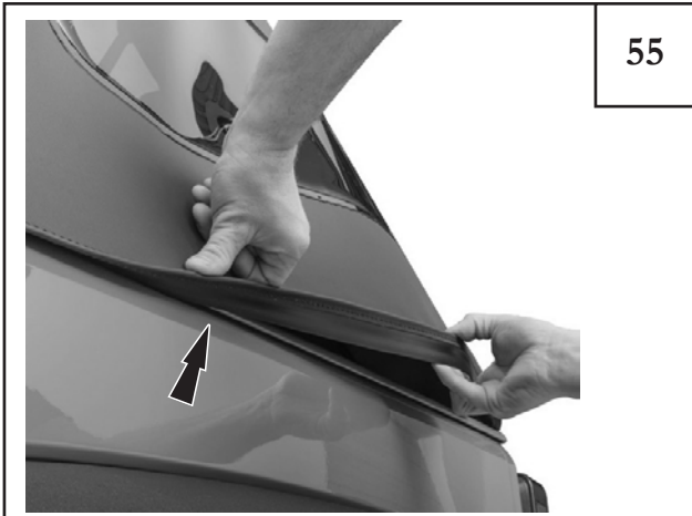
Slide lower rear qtr window channel into body tub rail as shown.
