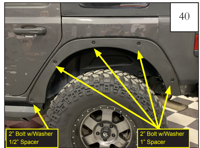
Use the noted hardware combinations to install the fender delete. Install from rear to front loosely. Tighten bolts once all 5 are installed.
