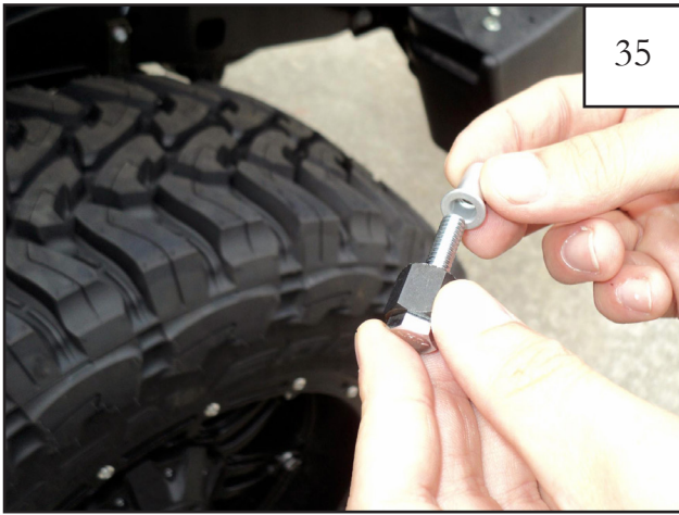
Place a rivnut (133606A) on the provided rivnut tool (133606H).
