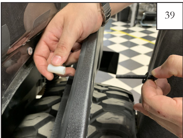
Install rear fender delete using 5 long bolts,(133606G) 5 washers (WA1-0029), and 5 spacers (1 short SP1-0004, and 4 long SP1-0005).
