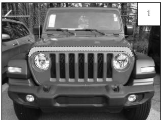
Prior to installation, wash the hood of vehicle and dry with a clean cloth. Use the alchohol pads to clean entire LEADING EDGE of hood. *NOTE: Temperature should be at least 60°F for proper tape adhesion.*
