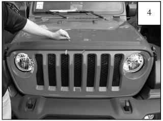
Begin removing tape liner starting with the passenger side Center Top. Grasp the free end and pull tape gently in 6" sections. Apply even pressure with opposite hand to the hood protector while pulling tape liner. Repeat for driver side. **NOTE:** You must apply even pressure from center section out to each end of part for proper adhesion to hood.
