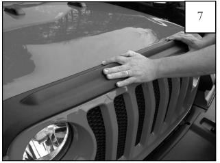
Apply firm pressure along all edges of hood protector to ensure adhesion of tape to hood surface. Installation is now complete. NOTE: Do not drive vehicle for 24 hours after installation. No not was vehicle for 72 hours after installation.
