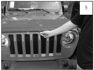
Using the same process, remove the tape liner from the center bottom of hood protector. Repeat for opposite side.
