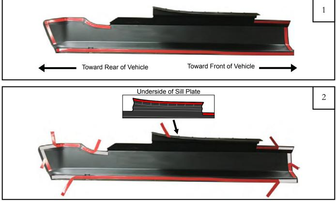
Open vehicle doors. Clean all dirt and debris from vehicle door sills and rocker panel. Use supplied alcohol wipes where part will attach.
