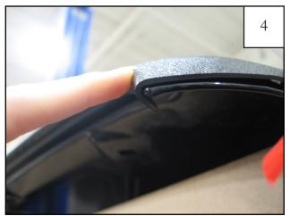
For proper alignment, check that edge of part is hooked over the edge of the hood along entire length of part. *NOTE: Hood will not close properly if part is not snug around the lip.*
