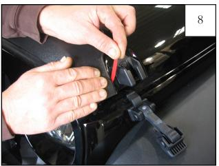
Pull the liner from the 1/4" tape on the driver's side of the vehicle.
