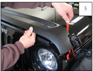
While pressing on the forward edge of the part, pull the 1/2" tape liner with the tab folded up in step 2. NOTE: Take care not to catch tape liner on other pieces of tape and accidentally pull their liners off as well.
