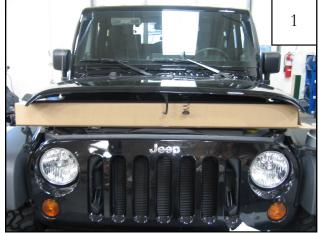
Open front hood. Using box parts came in, prop hood open. Clean all dirt and debris from hood then use supplied alcohol wipe where part will be. *NOTE: Temperature should be at least 60°F for proper tape adhesion.*
