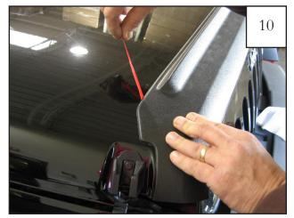
Take the tab of the remaining 1/4" tape strip and pull tape liner. While pulling liner, press on part as was done for first strip of tape liner.
