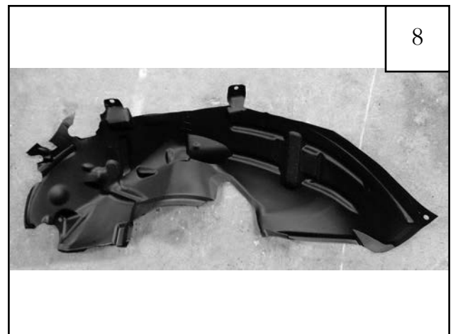
Splash shield properly trimmed.
