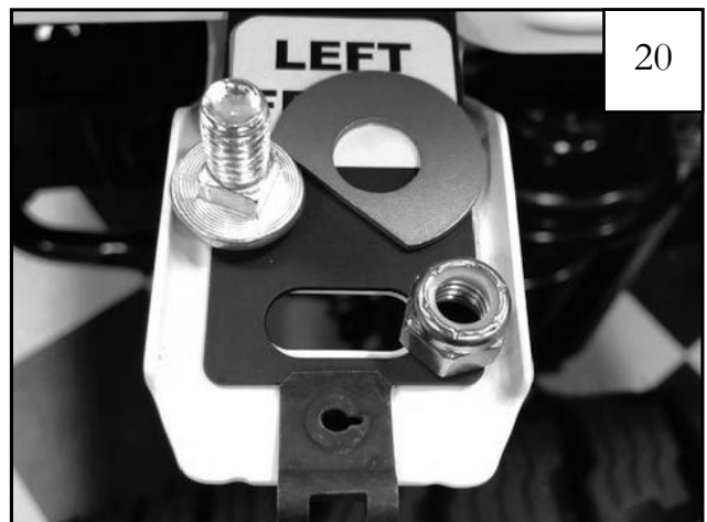
Attach both flanges of the support bracket to the existing factory fender support using a carriage bolt, anti-rotating clipped washer and nylock nut.
