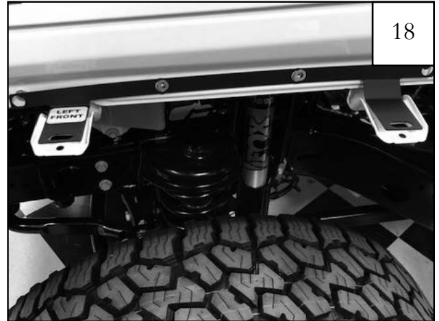
Position support brace along the top edge of fender opening, aligning with the existing factory supports.
