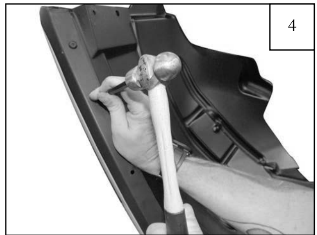
Use a punch or drill with 5/16" bit to drill through eight plastic rivets along edge of flare/splash shield. Discard flare. Save splash shield for reinstallation.
