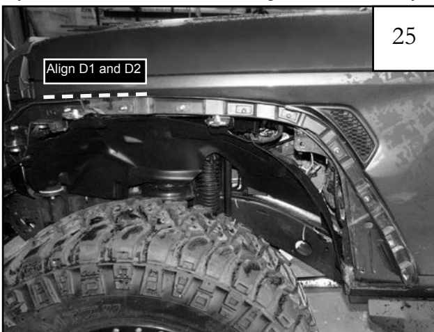
Ensure that inner pieces D1 and D2 are aligned together properly, and tighten all allen head bolts.
