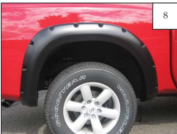
Passenger Side Flare: Completed rear flare installation.
