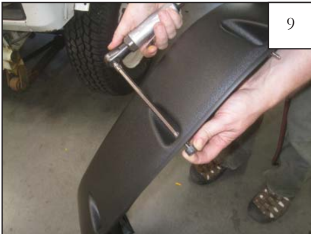
At each flare pocket, insert a Screw (SW1-0045) and run it into a Spacer (SP1-0009) until snug with the flare plastic. Use a 5/16" socket and 6" extension to prevent marring flare plastic. Wrap a layer of masking tape around Torx Bit (SW1-0052) to help it stay in the socket.
