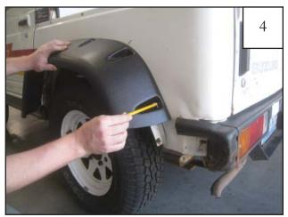
Hold rear flare in position on fender and, using a grease pencil, mark each hole location on sheet metal.
