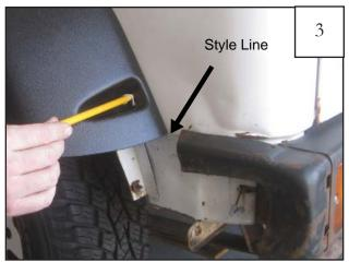
For rear of rear flare, use style line of vehicle as guide for where flare should line up. If there is a rear bumper endcap extending above this line then it will need to be trimmed.
