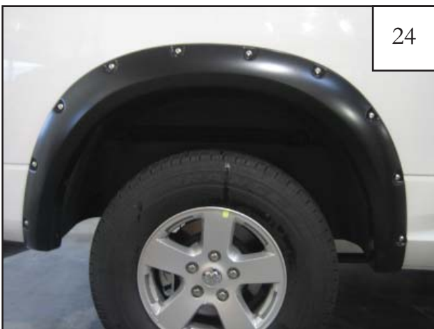
Completed rear flare installation.
