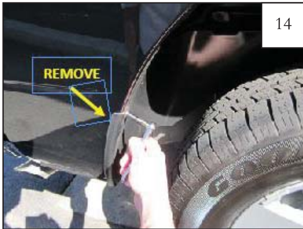
2012 -2014 Models Only (Optional): If you encounter a fit problem, remove inner piece at bottom rear and front of wheel well.
