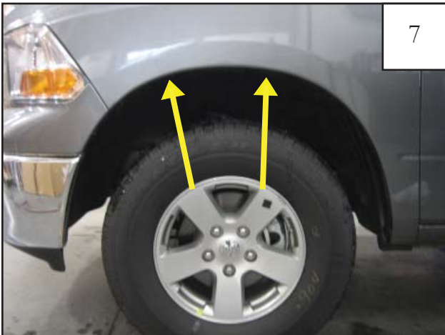
Two Clip locations. See step 9. NOTE: There are two factory holes near the rearward arrow. The correct hole for install is the one more toward the front of the vehicle.
