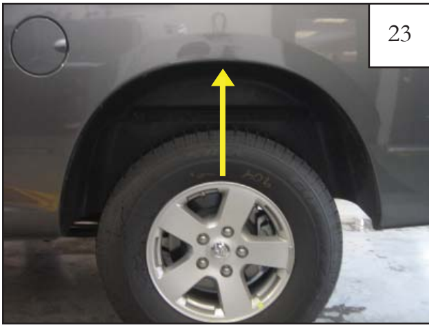
Install #10 U-Clip in this location. See step 25.
