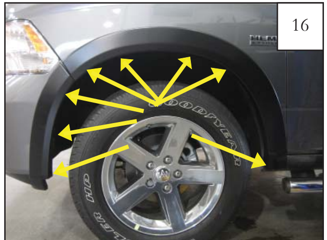
PLASTIC BUMPER ONLY: Press firmly on flare and tighten all screws.
