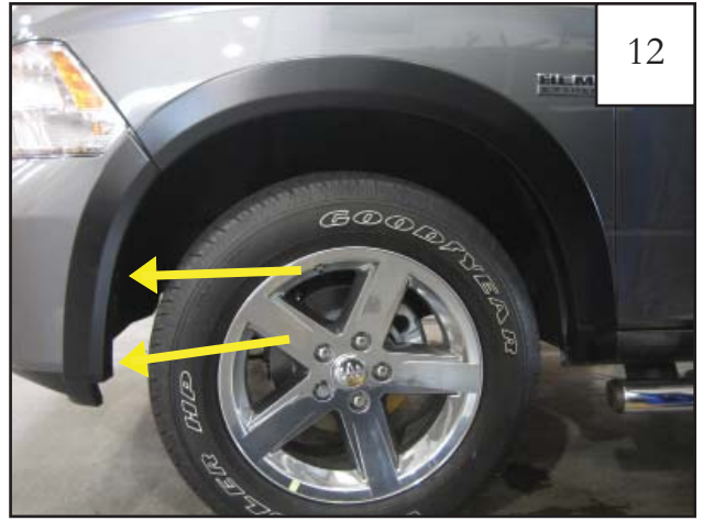
PLASTIC BUMPER ONLY: Additional supplied screw locations.
