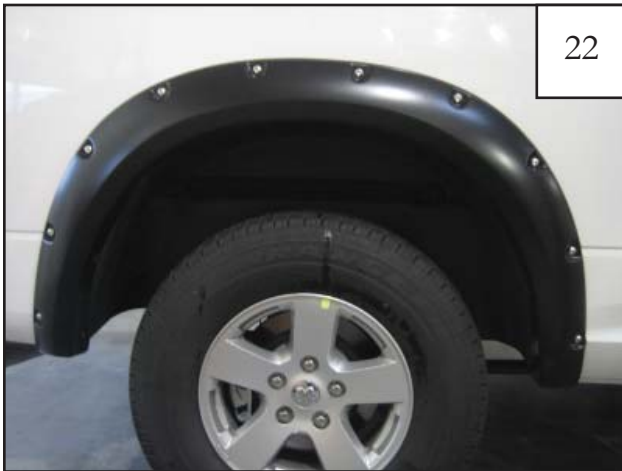
Completed rear flare installation.
