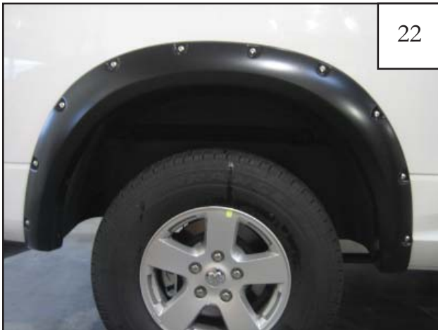
Completed rear flare installation.
