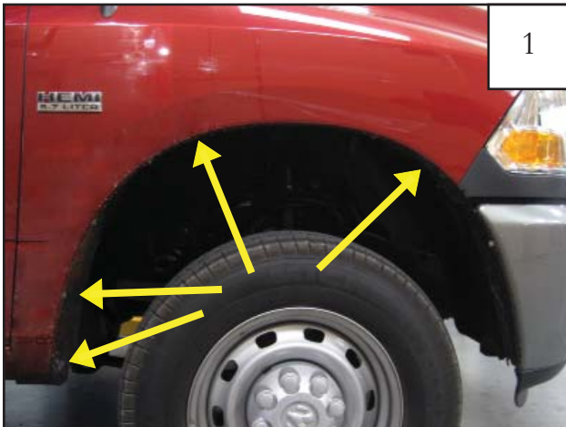
Remove four factory installed screws with 8 mm socket wrench. Save screws for reinstallation.
