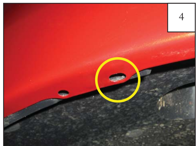
At location in step 3, there is a lip with two factory holes. One hole is a circle and one is an oval. The 1"x1.5" Black Tab and #10 U-Clip will be installed over the oval. The oval is the hole more toward the front of the vehicle.
