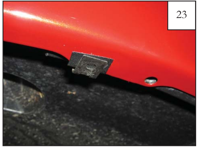
Install #10 U-Clip over 1"x1.5" Black Tab.
