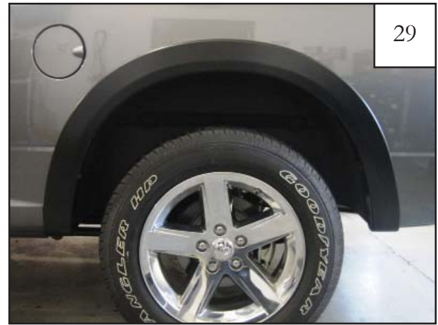
Completed rear flare installation.
