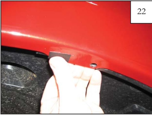
Install 1"x1.5" Black Tab over existing factory hole.
