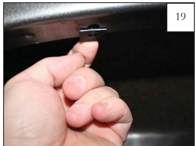
Install Clip (CL1-0022) over existing hole.
