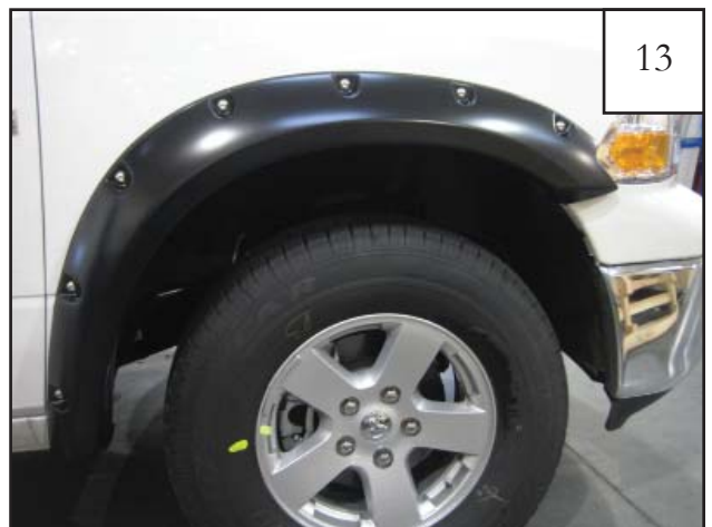
Completed front flare installation.
