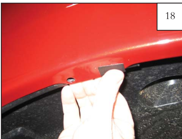
Install plastic tab over existing factory hole.
