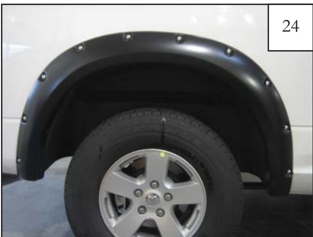
Completed rear flare installation.
