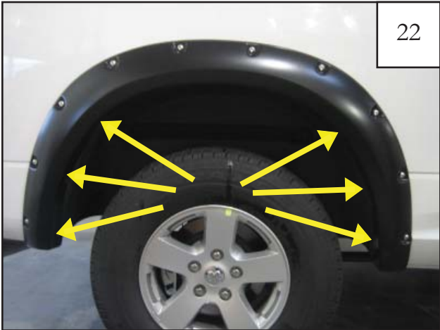
Hold flare in place start six supplied screws using an Phillips Head Screwdriver. Do not tighten.
