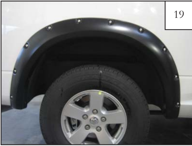
Completed rear flare installation.
