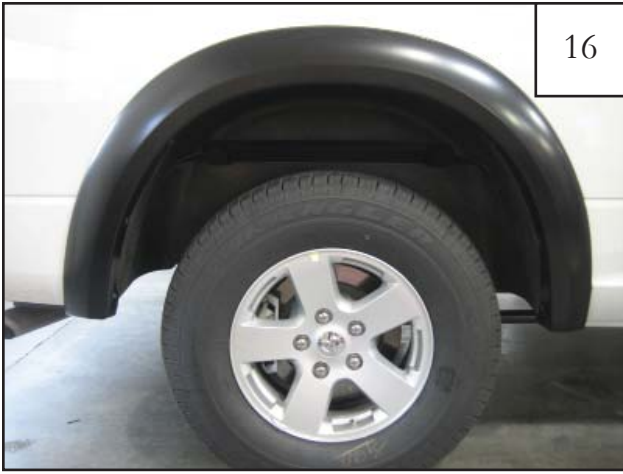
Completed rear flare installation.
