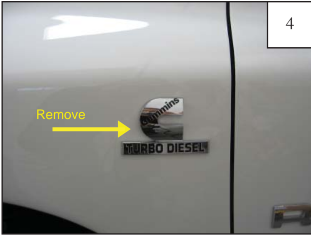
If there is a Cummins logo on the vehicle, it must be removed prior to installing front flares.
