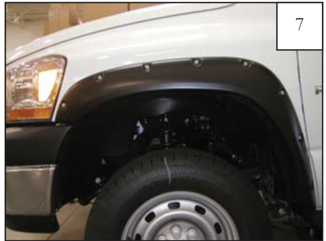
Make sure flare is correctly positioned on vehicle. Tighten all screws.
