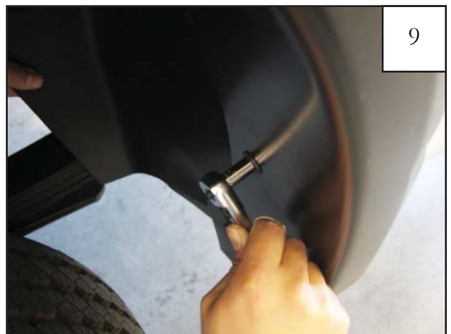
Holding flare in position on fender, reinstall screws removed in Step 8. Do not tighten. (An awl may be used to align the threaded clip with holes in flare and fender lip) Note: Make sure screws engage in splash shield.
