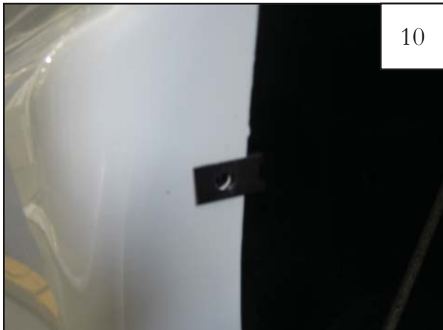
Install Clip (CL1-0011) over existing factory hole.
