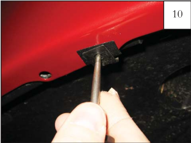
Using an awl or similar pointed tool, poke a hole through Tab (MT1-0014) using the Clip (CL1-0022) hole as a guide.
