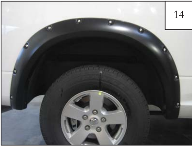
Completed rear flare installation.
