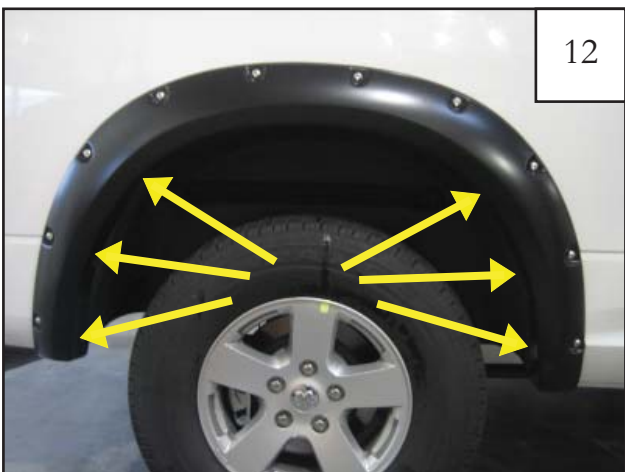
Hold flare in place while you start six supplied screws (SW1-0056) using a phillips screwdriver. Do not tighten.
