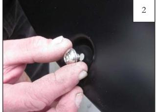
Put each Bolt/Washer combination through a pocket hole in the flare, Bolt head and Washer on the outside.
