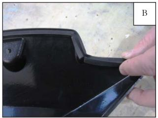
At the inward, right angle curve in the flare, cut a notch in the edge trim so when you apply along the part, the edge trim doesn't stretch.
