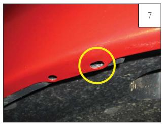
At location in step 6, there is a lip with two factory holes. One hole is a circle and one is an oval. The Tab (MT1-0014) and Clip (CL1-0022) will be installed over the oval. The oval is the hole more toward the front of the vehicle.
