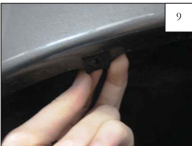
Install #10 U-Clip (CL1-0022) over existing factory holes.
