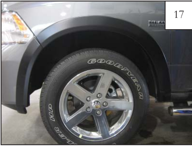
PLASTIC BUMPER ONLY: Completed front flare installation.
