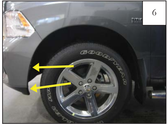
PLASTIC BUMPER ONLY: Remove two factory installed tufflocks.
