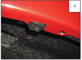
Install speed clip over plastic tab.
