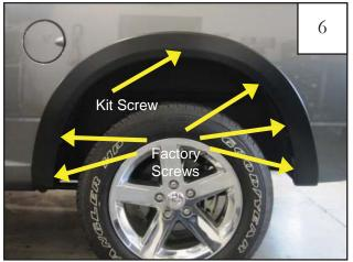
Kit supplied screw and factory installed screw locations. See steps 7 & 8.
