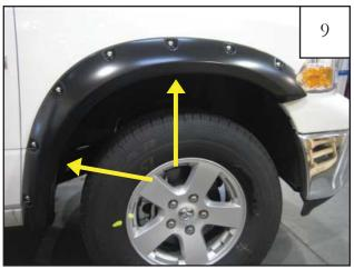
Hold flare to vehicle and start the kit supplied Screws (SW1-0056) with a Phillips screwdriver. *Do not tighten*.
