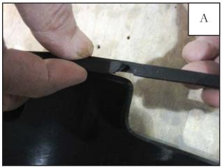
Start at the rearward end of the front flare and work toward the front. At the outward, right angle curve in the flare, cut a V out of the edge trim so when you wrap around the part, the edge trim doesn't bulge.
