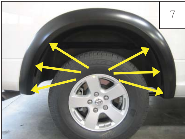
Hold flare in place while you start six factory screws using an 8 mm socket wrench. Do not tighten.
