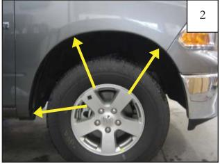
Remove three factory installed screws with 8 mm socket wrench. Save screws for reinstallation.
