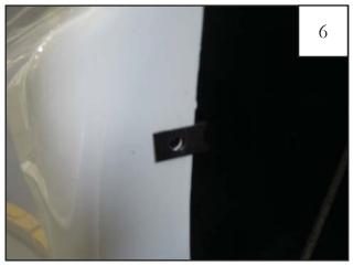
Install Clip (CL1-0011) over existing factory hole.
