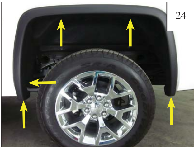
Remove fasteners from factory wheel arch molding using a T-15 Torx Bit for upper and lower wheel well fasteners and a 10mm deep socket and wrench for the lower 2 locations. Save the two lower fasteners for re-installation.
