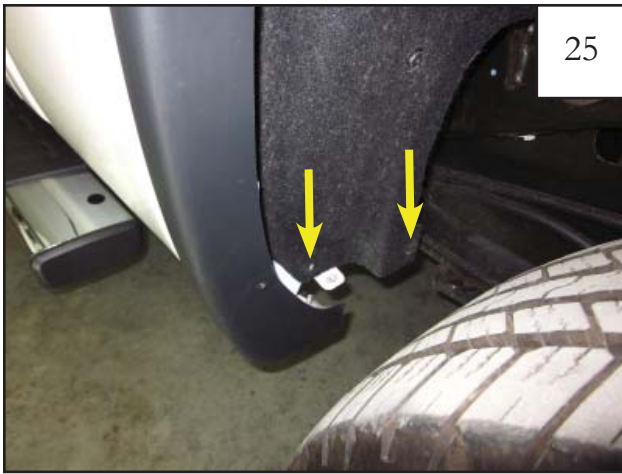
Re-install two factory screws into wheel well liner.
