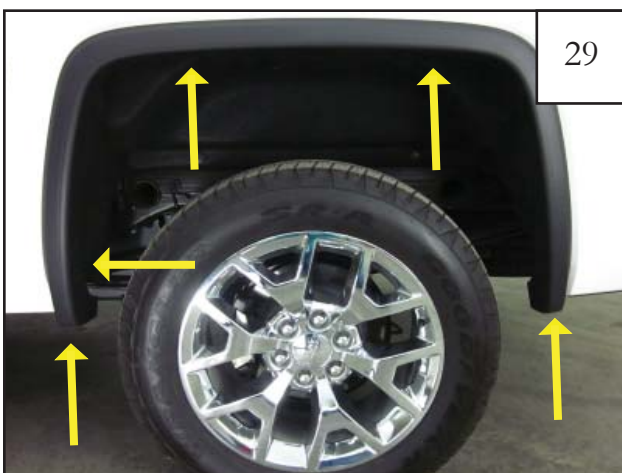
Remove fasteners from factory wheel arch molding using a T-15 Torx Bit for upper and lower wheel well fasteners and a 10mm deep socket and wrench for the lower 2 locations.
