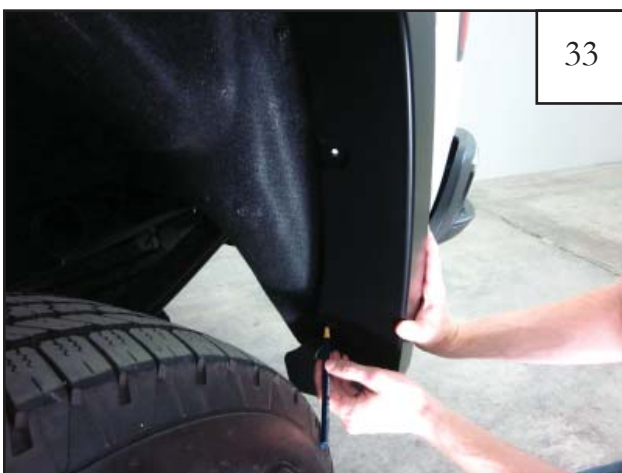
33 Using a grease pencil or marker, hold flare in place on vehicle and mark hole locations for drilling (3 places).
