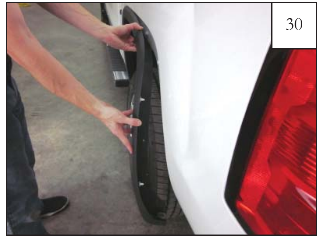
30 Starting at the lower rear end of the factory flare, firmly grip part and pull to remove from vehicle. Note: You will hear popping sounds as the factory fasteners release from vehicle. This is normal.
