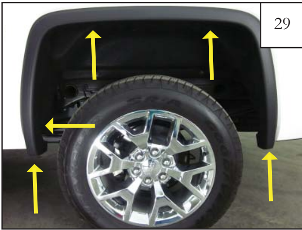
29 Remove fasteners from factory wheel arch molding using a T-15 Torx Bit for upper and lower wheel well fasteners and a 10mm deep socket and wrench for the lower 2 locations.
