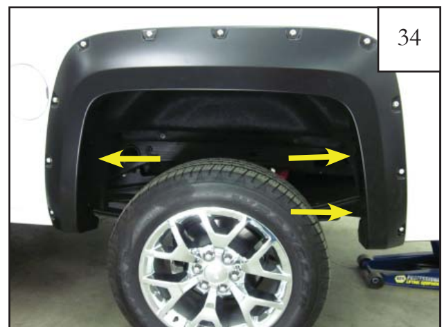
34 Hole locations to be marked for drilling.
