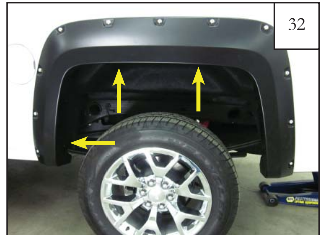
32 Hold rear flare up to wheel well to confirm fit. While holding flare on vehicle, install supplied screws (SW1-0056) into the 2 upper and 1 lower factory hole locations. Do not fully tighten at this time.
