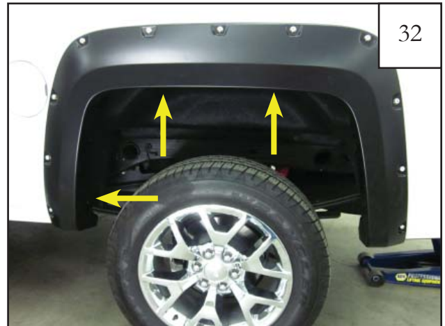
Hold rear flare up to wheel well to confirm fit. While holding flare on vehicle, install supplied screws (SW1-0056) into the 2 upper and 1 lower factory hole locations. Do not fully tighten at this time.
