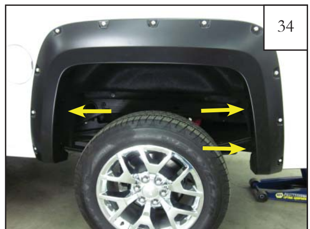
Hole locations to be marked for drilling.
