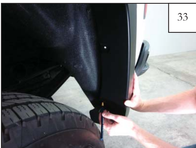
Using a grease pencil or marker, hold flare in place on vehicle and mark hole locations for drilling (3 places).
