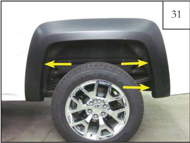
Hole locations to be marked for drilling.
