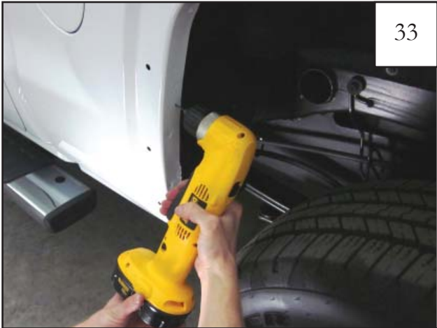
Using a 3/32" drill bit, drill pilot holes through sheet metal at the marks made in Step 30.
