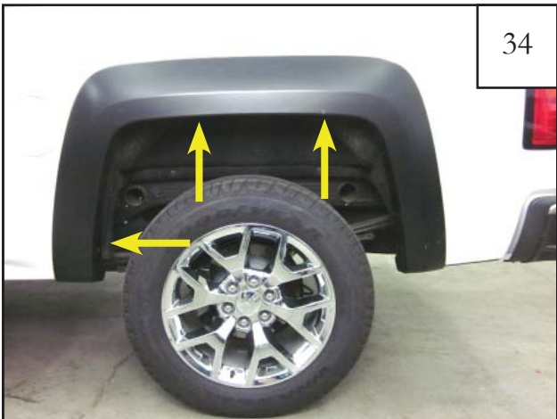
While holding flare on vehicle, install supplied screws (SW1-0056) into the 2 upper and 1 lower hole locations. Do not fully tighten at this time.
