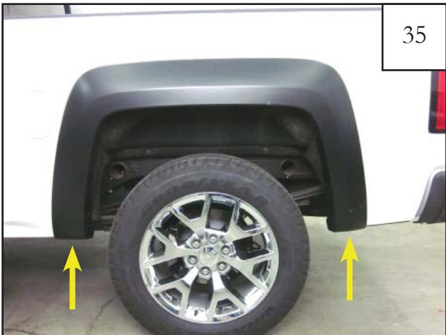
Reinstall the lower 2 factory fasteners removed in step 24 using a 10mm deep socket and wrench.
