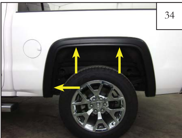
While holding flare on vehicle, install supplied screws (SW1-0056) into the 2 upper and 1 lower factory hole locations. Do not fully tighten at this time.
