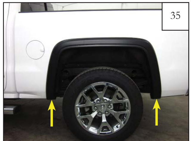
Reinstall the lower 2 factory fasteners removed in step 24 using a 10mm deep socket and wrench.
