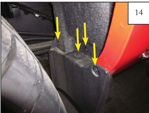
Using a T-15 Torx bit socket wrench, remove the four factory screws from the factory forward splash guard. Remove splash guard and discard.
