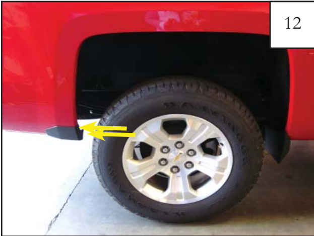
Using a T-15 Torx bit socket wrench, remove factory installed screws from factory rear mudguard. Discard screws.
