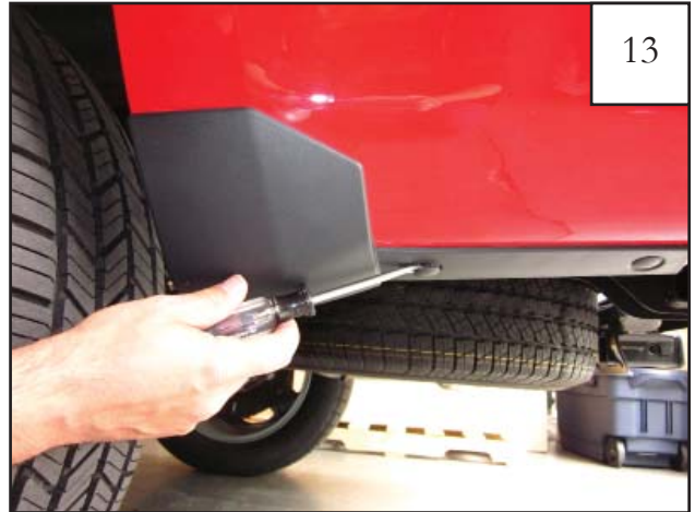
Using a pry tool, remove factory retainers in bottom of factory rear mudguard. Remove mudguard and discard.
