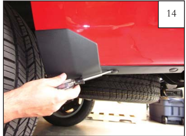
14 Using a pry tool, remove factory retainers in bottom of factory rear mudguard. Remove mudguard and discard.
