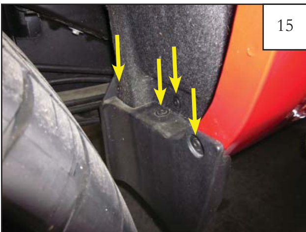
15 Using a T-15 Torx bit socket wrench, remove the four factory screws from the factory forward splash guard. Remove splash guard and discard.
