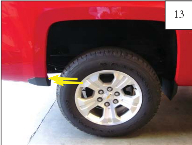
13 Using a T-15 Torx bit socket wrench, remove factory installed screws from factory rear mudguard. Discard screws.
