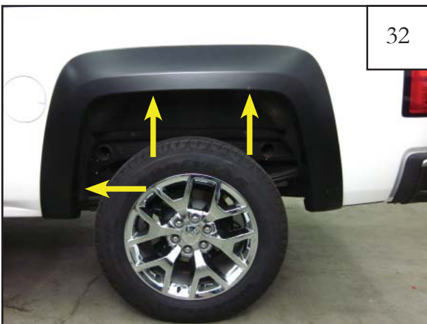
While holding flare on vehicle, install supplied screws (SW1-0056) into the 2 upper and 1 lower hole locations. Do not fully tighten at this time.
