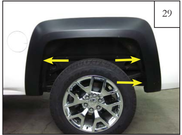
Hole locations to be marked for drilling.
