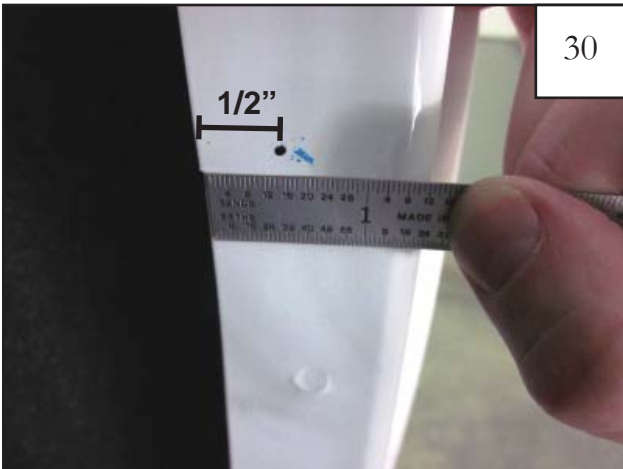
Remove the flare. At the marked locations made in Step 28, measure inward 1/2" from the inside edge of the fender and make a new mark. This is the mark to be drilled.
