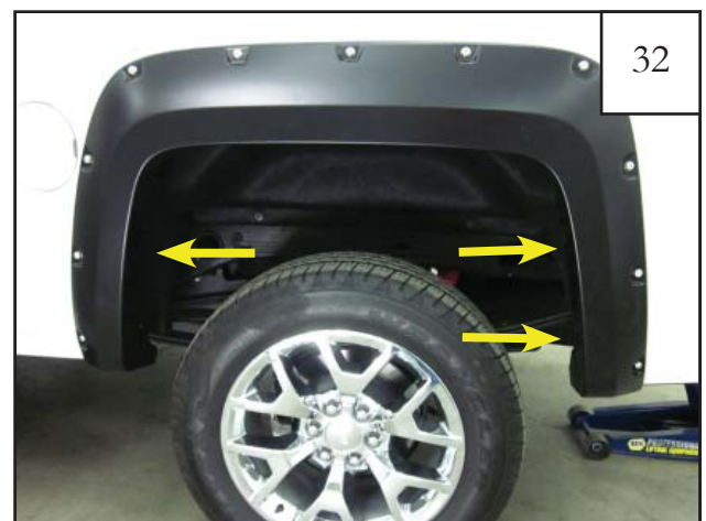
32 Hole locations to be marked for drilling.
