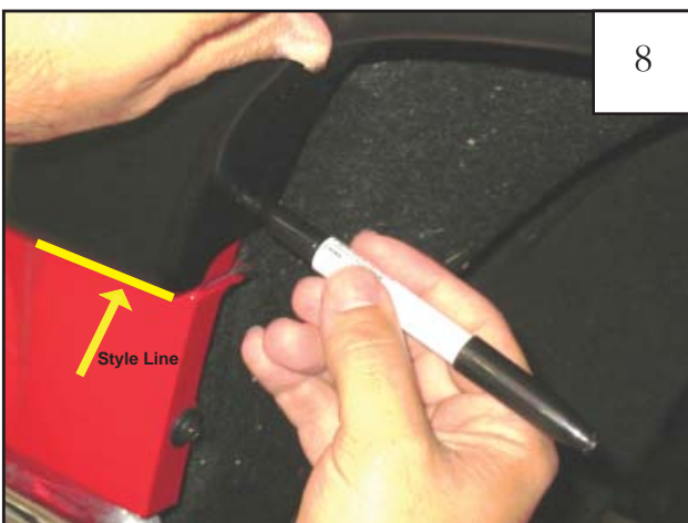
While holding the flare firmly in position, mark the remaining five hole locations with a grease pencil or sharpie, using the holes in the flare as a guide. Press inward firmly on the flare above each hole location before making each mark, this will ensure proper fit. See next step.
