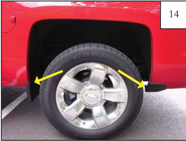
Using a T-15 Torx bit socket wrench, remove factory installed screws. Discard screws.
