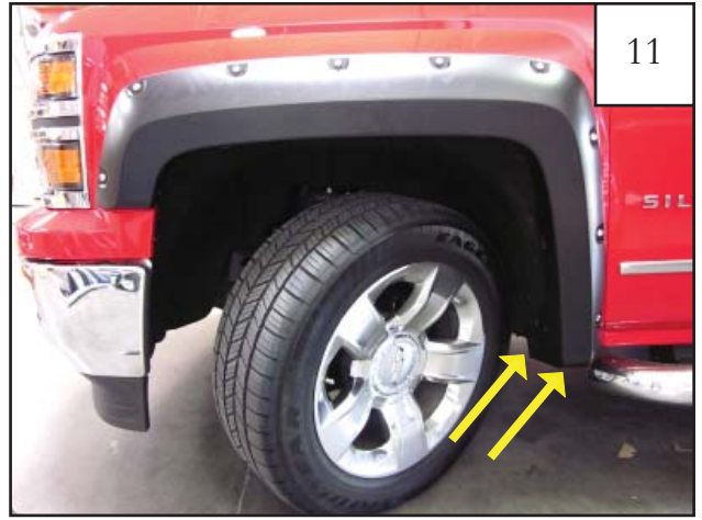
Locate flare into position on vehicle. Install supplied screw (SW1-0056) through two bottom rear holes in flare and into factory hole in rear of wheel well.
