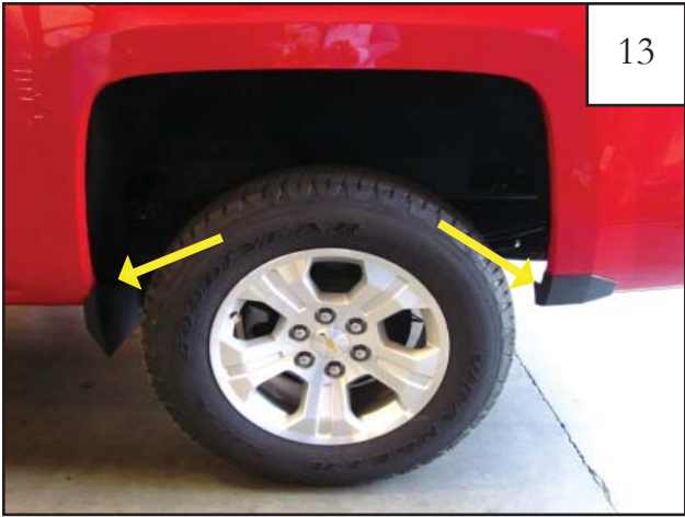
Using a T-15 Torx bit socket wrench, remove factory installed screws using. Discard screws.
