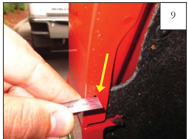
Remove the flare. At the marked location made in Step 7, measure inward 10mm from the edge of the fender. These are the marks to be drilled. Note: Marks at 10mm may be on either side of the first mark.
