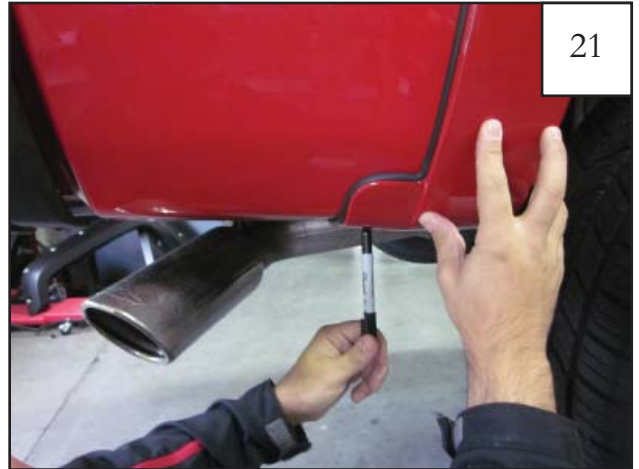
Using a grease pencil, mark the rear bottom fastener using the flare as a guide.
