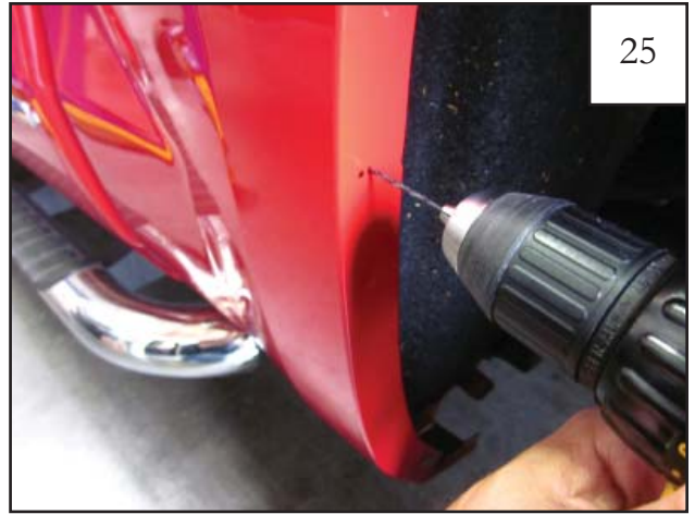
Using a 3/32" drill bit, drill pilot holes at the marks made in Step 24.
