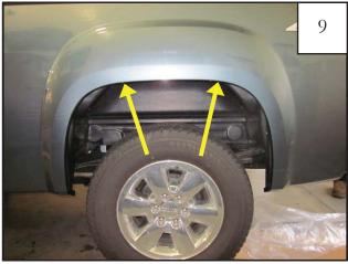
Remove factory mudflap if applicable. Remove and discard two factory installed plastic retainers in top (outer) hole locations of sheet metal (ignore center location). *NOTE: Not all vehicles have plastic retainers installed.*
