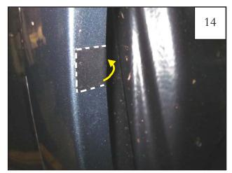
Center a supplied Tab (MT1-0014) over the four marks made in Step 12, aligning edge of Tab with outside edge of fender lip. Fold around back edge of fender lip and press firmly to adhere.
