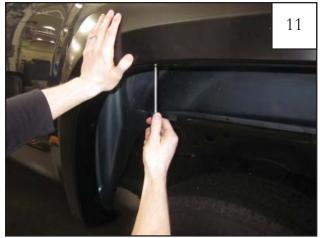
Align flare on vehicle and start a supplied screw (SW1-0058) through the two uppermost holes in the flare and into each clip installed in Step 10. *DO NOT FULLY TIGHTEN SCREWS AS THEY WILL BE UNINSTALLED*
